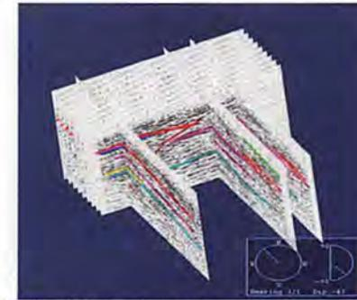
Fig.10. 3D data volume and several In-Line sections.
