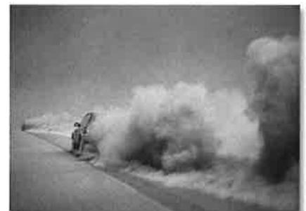
FIGURE 15 RESUSPENSION OF TEPHRA SURFACE LAYERS BY VEHICLES
